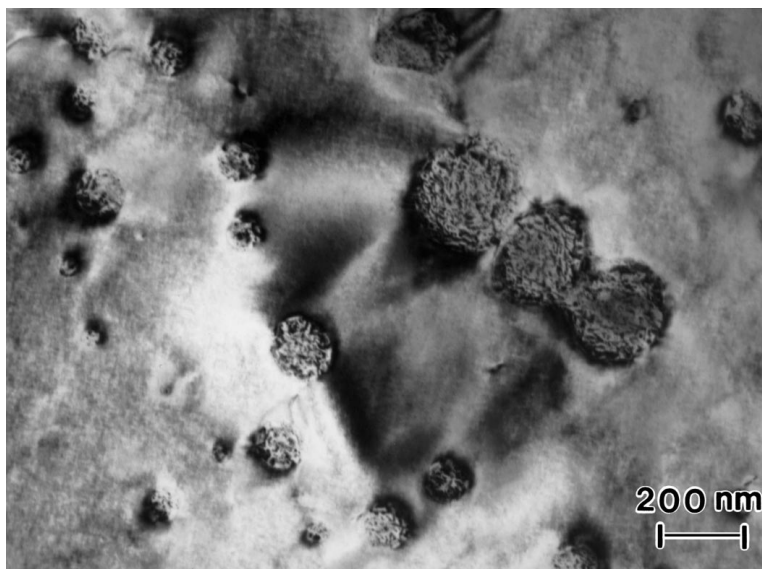
Figure 9 Intradendritic \alpha -Cr precipitates in the as-cast Ni-28 at % Al-18 at % Cr-6 at % Ti alloy, imaged in BF.
