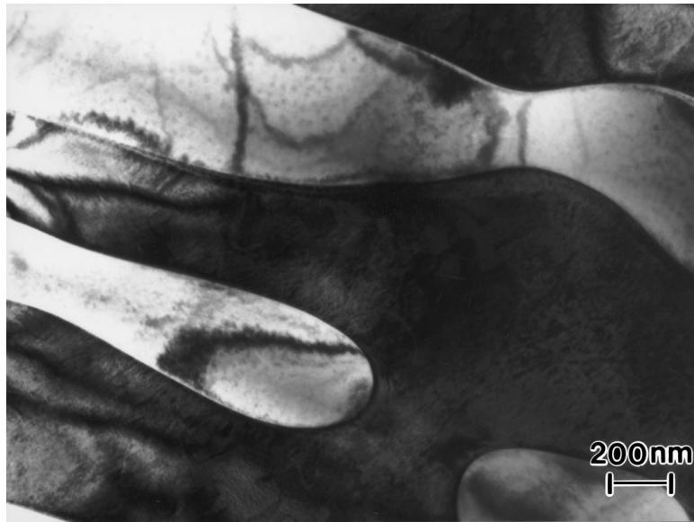
Figure 4 BF micrograph showing the \beta' - \alpha eutectic present in the as-cast Ni-26 at % Al-19 at % Cr-8 at % Ti alloy. In this image, the \alpha -Cr appears as the lighter toned features and the \beta' as the darker toned regions.
